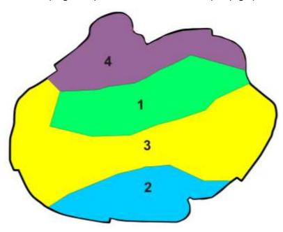
**Figure: 1.** Scheme of dividing the working area of the Muruntau open-pit mine into active and passive parts: 1 - non-working open-pit side; 2 - temporary rear sight; 3 - the main working area; 4 - "North Board".
